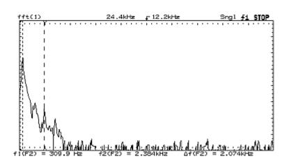
Even though the signal amplitude was considerably less for the fourth "bounce", the FFT function could extract the resonant frequency of the metal shield, and again identified it to be about 2.4 kHz.
