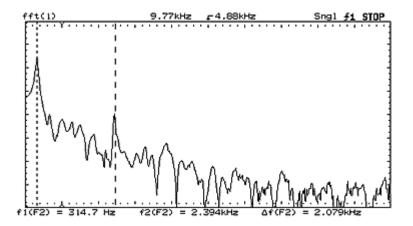
Clearly, the speaker cone resonance was about 315 Hz, and the FFT now allowed me to see the "klink" frequency: about 2.4 kHz.
