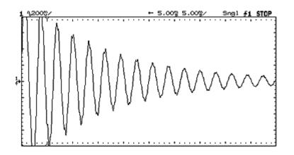
With the time base set at 5ms/div (ten times faster than it was set when I actually acquired the waveform), I could read the cone's resonant frequency. I couldn't see the "klink" frequency in the decaying waveform, so I put the scope in FFT mode:
